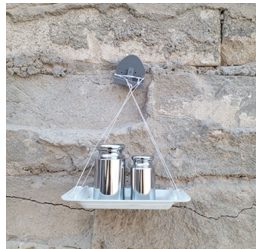
Fig. 15. One fishing-hook that hanging on the concrete wall with 1.5 Kg payload (Sliding moment).
