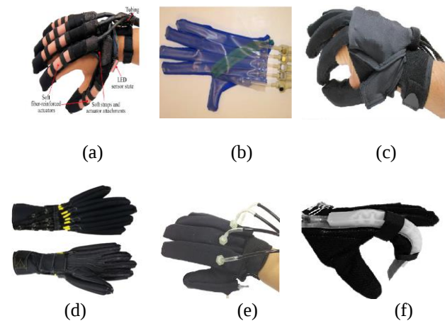
Fig. 3: Robotic Glove Based on Pneumatic Actuation (a): Penu Glove [1], (b): soft robotic glove [6], (c): Penu robotic glove [7], (d): soft pneumatic actuator [1], (e) inflatable actuators [8], (f): AirExGlove [17].
