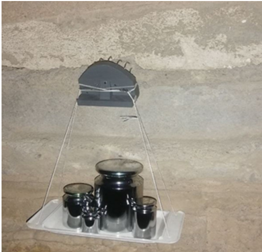
Fig. 16. Seven fishing-hook that hanging on the concrete wall with 3.75 Kg payload.
