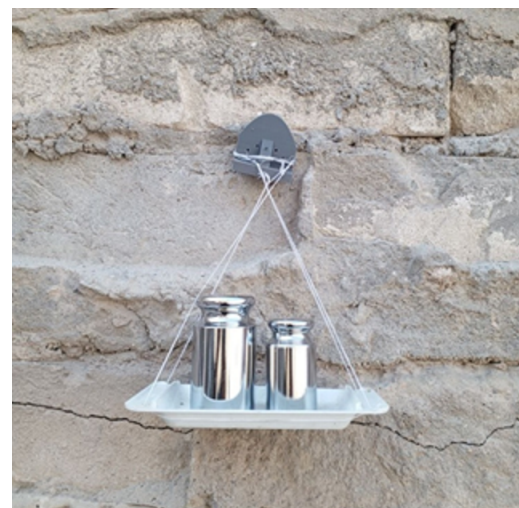
Fig. 15. One fishing-hook that hanging on the concrete wall with 1.5 Kg payload (Sliding moment).
