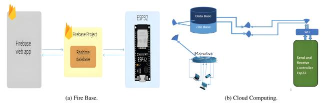
Fig. 6. Fire base and cloud computing.
