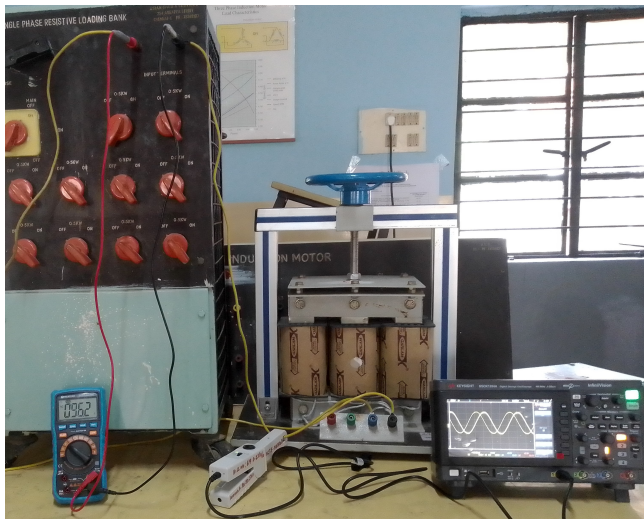
Fig. 9. Hardware implementation of the proposed system with R-L load
