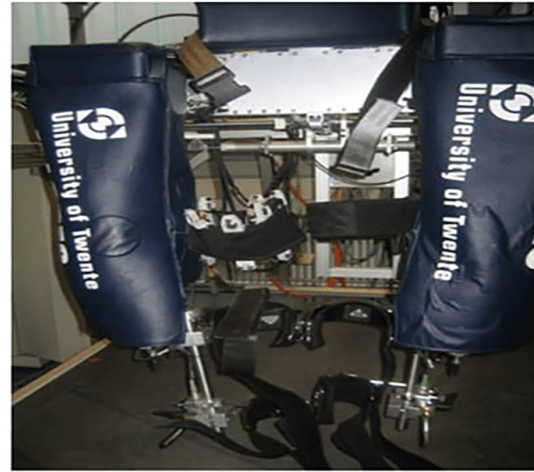
Fig. 21. The sensorized fastening belts and the Lopes exoskeleton for lower-limb rehabilitation [12].
