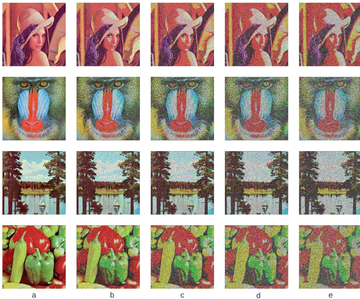
Fig. 22. Decrypted images with different standard deviation values of Gaussian noise. (a) \sigma = 0.5 , (b) \sigma = 5 , (c) \sigma = 10 , (d) \sigma = 15 and (e) \sigma = 20 .
