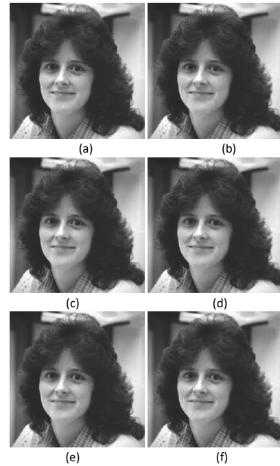
Fig. 3. Sample 2 image from custom-built database/proposed LSB technique. (a) Original cover image, (b) Stegoimage with message size of 6KB, (c) Stegoimage with message size of 8KB, (d) Stegoimage with message size of 10KB, (e) Stegoimage with message size of 14KB, (f) Stegoimage with message size of 16KB.
