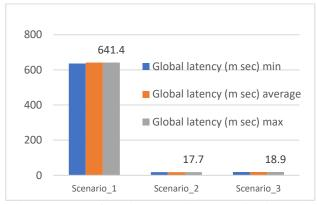
Fig. 7: Latency of 16 video surveillance applications with different scenarios.
