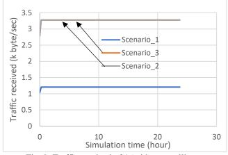
Fig. 9: Traffic received of 16 video surveillance applications with different scenarios.
