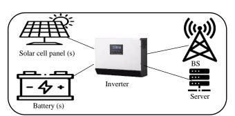
Fig. 2: Green WiMAX infrastructure self-powered supply.
