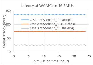
Fig. 5: Global latency of WAMC application for 16 PMUs.
