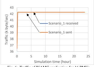
Fig. 6: Traffic of WAMC application for 16 PMUs.
