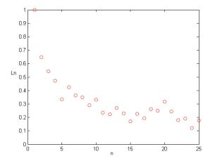
Figure 4. Trend of the Ln parameter for the Kaplan test of a random signal with with the same mean and variance of the filtered signal
