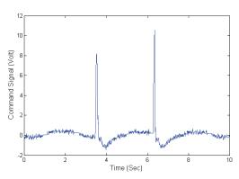
Figure 4. Output signal of the explicit model predictive controller which is applied to DC motor.
