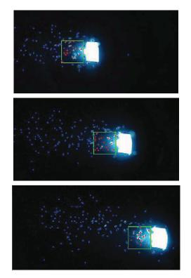
Figure 4. Frames showing motion control of an Artemias population through a robotic system.
