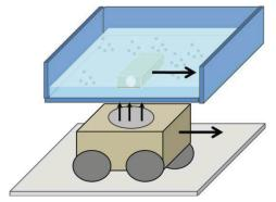
Figure 3. Schematic of the robot used for controlling Artemias motion.
