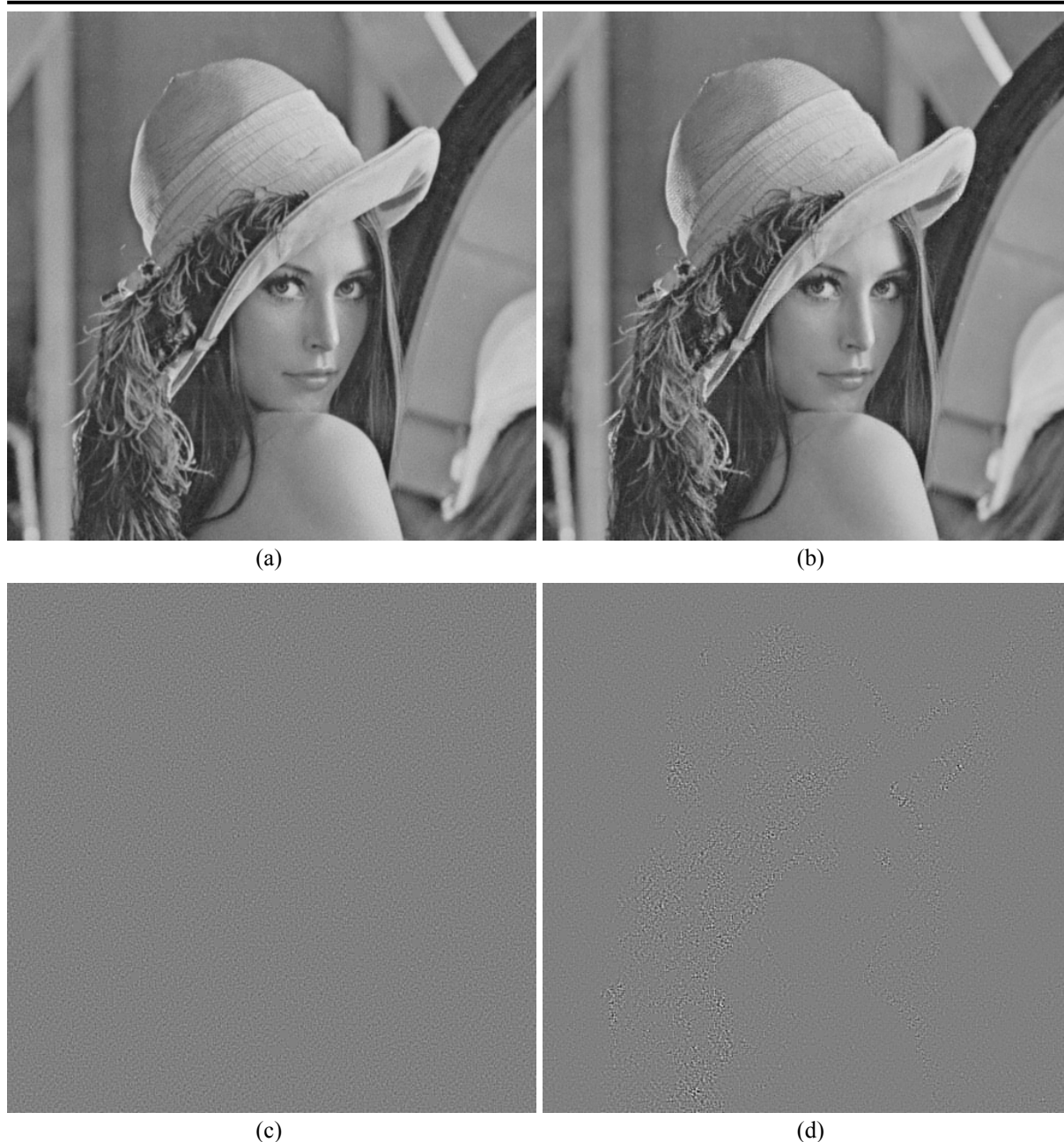
Fig. 6. Two differently marked versions of the test image using (a) the nonadaptive spread transform QIM marking technique, and (b) the proposed partially host-adaptive baseband-spread transform QIM marking technique, along with the watermarks embedded within, shown in (c) and (d), respectively.
