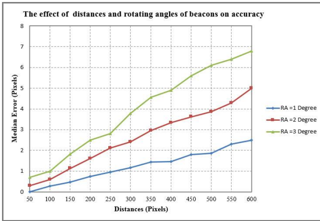
Fig. 27. Median error estimation of the robot position with 10 pixels radius vs. distances, for several values of the rotating angle of beacons.
