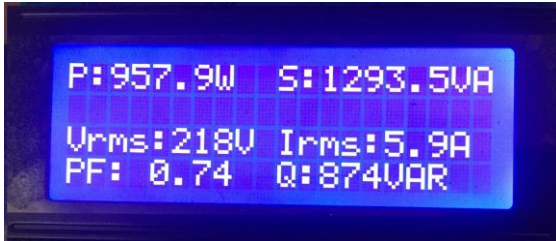
Fig.16. Condition of Load before APFC
