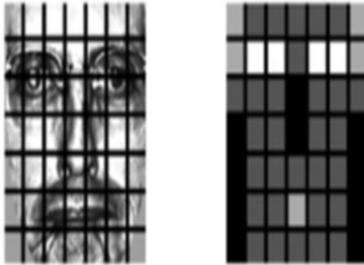
Figure 5. A preprocessing of face mask image example divided into 49 windows
