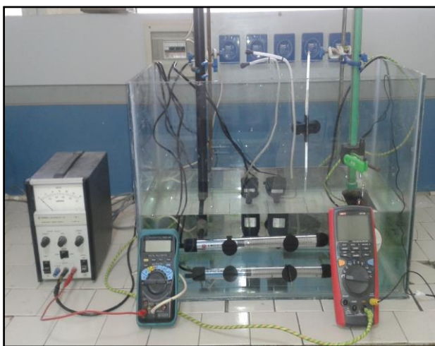
Fig. 2 Photo of the Installed ICCP System.
