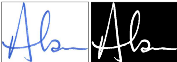
Fig. 4. Two images for the same signature. On the left: the original signature image. On the right: the binary format of the image.
