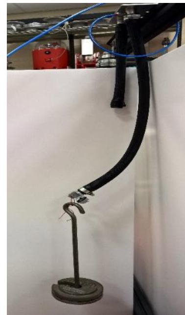
Fig. 4. A 30 cm SBCA at 300 kPa and loaded by 1.0 kg.
